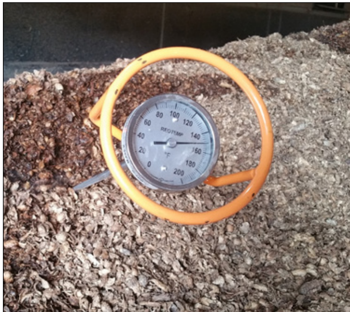
Fig. 6. Temperature probe in windrow (Source: Gary Flory, 2018).
